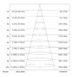
Diagram for RC100LEDSQ-01 in 4000K. Other diagrams available on request
