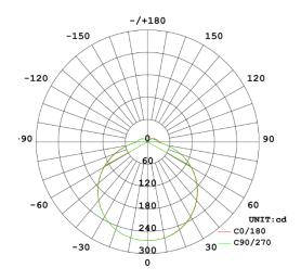
Diagram for RC100LEDSQ-01 in 4000K. Other diagrams available on request
